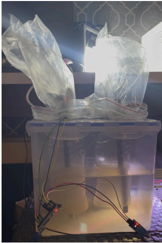
Fig 13. Electrolytic Cell Setup with the Device for Measuring Experimental Conditions and Hydrogen Concentration
